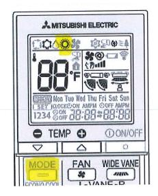
Set the CERV 2° higher than the heat pump – this allows the CERV to act as the primary heat source. If you want to change the temperature, adjust both the heat pump and CERV to maintain the 2° difference. Set the CERV cooling set point at 90° to prevent any cooling from occurring.
