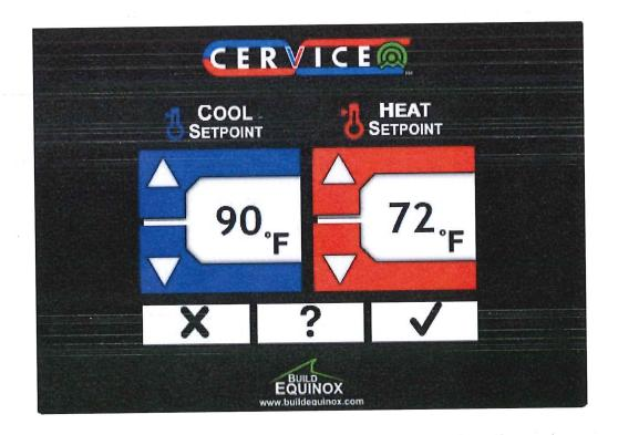
**COOLING SEASON**: <u>Set the CERV at your desired temperature</u> (for example, 74°). Set the heating set point to 55° so that the heat never comes on. Try cooling with just the CERV and keep your heat pump off to save energy.
