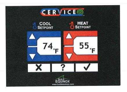
home cool or dry enough, turn on the heat pump and make sure it is in cooling mode by pressing the mode button until the snowflake icon appears at the top of the screen. Set the heat pump 2° higher than the CERV. If you want to change the temperature, adjust both the heat pump and CERV to maintain the 2° difference.
